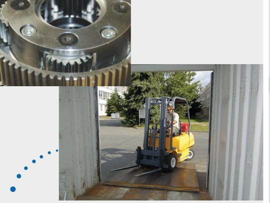
The **D** (**G**) 12 - 20 series trucks are intended particularly for work in storage spaces, containers and wagons, to which the low height of the protective frame and the lifting device with a big free lift are adapted. All the trucks of this series are approved for operation on roads and at the Client's wish they can be provided with the obligatory outfit.
