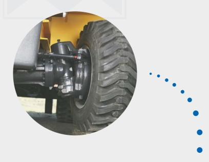
The clutchable KANZAKI rear axle drive ensures an easy recovery on soft ground or in winter months for the DV 35 T series trucks.
