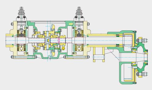
The possibility to use the quality renowned KNOTT plate brakes offers an option to increase the braking effect and its adjustment acc. to requirements of the most demanding clients and their facilities. The brakes have a permanent oil bath, which provides them with a long operating life.
