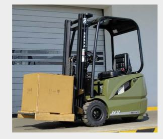
The new accumulator trucks of a contemporary construction have a lower operating cost compared to engine - driven trucks. For 5 years of operation the approx. 50%.
